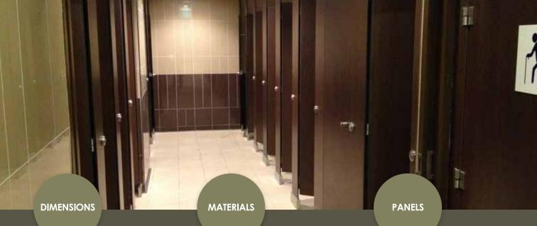
Suggested cubicles' 2000mm overall height, measured from the finished floor level to the top of the head rail includes a 150mm floor clearance. Its width and depth are tailored to meet your preferences and to adapt to individual site conditions.
